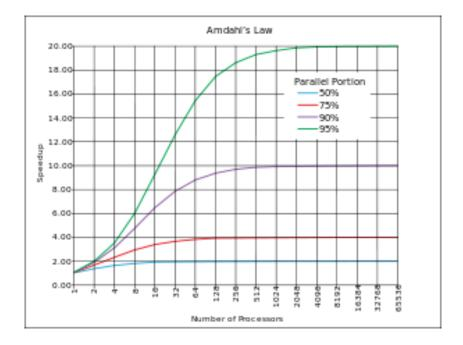
The speedup of a program using multiple processors in parallel computing is limited by the sequential fraction of the program. For example, if 95% of the program can be parallelized, the theoretical maximum speedup using parallel computing would be 20× as shown in the diagram, no matter how many processors are used.
