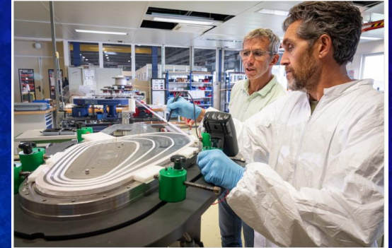
Luca Bottura, project lead of GaToroid, and Gregory Maury from the TE/MS-SMT section are working on winding a coil of the demonstrator for GaToroid.
