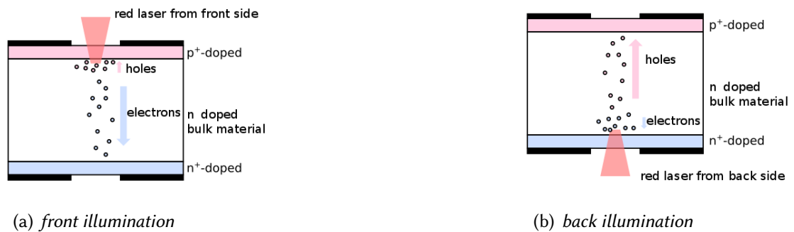
Figure 3: TCT measurements illustrating the two illumination methods and the corresponding charge movement in the sensor bulk.
