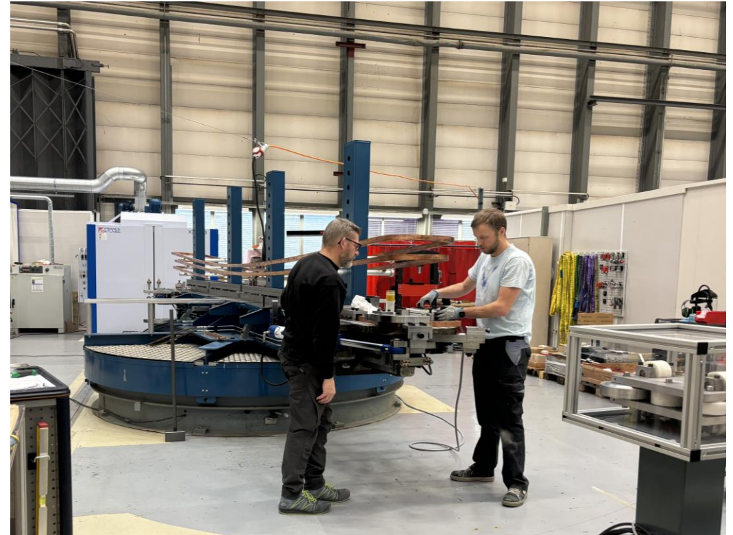
Winding machine operated in building 181, by TE/MS-C-NCM, for the manufacturing of the resistive coils of the SPS MBB magnets (coil are 6.5 m long)
