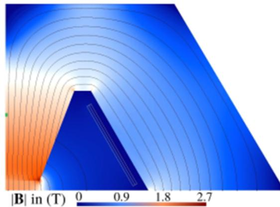
**Fig. 6.1.17:** MAP design with increased coil length and gap dimensions 30x100mm
