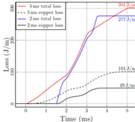
**Fig. 6.1.20:** Resistive and total loss evaluation for two cycle alternatives with the same ramp time of 1 ms, but either 2 ms or 5 ms total time, see Fig. 6.1.14. The geometry of the modified US-MAP dipole, see Fig. XXX, was used for this calculation.
