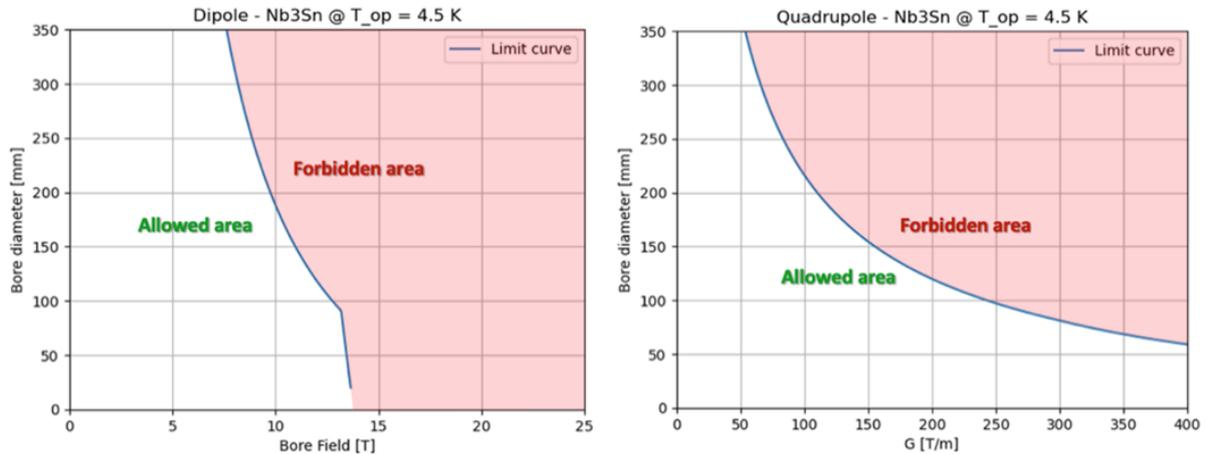
**Fig. 6.1.25:** A-B plot for dipoles and A-G plot for quadrupoles built with Nb3Sn and operated at 4.5 K.
