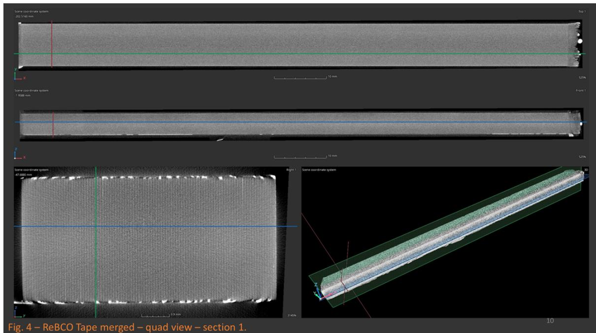
**Fig. 6.1.13:** Tomography of a stack of ReBCO tapes soldered under vacuum – negligible porosity achieved.
