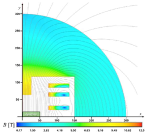
Fig. 6.1.24: Conceptual design of a 10 T HTS, 30 mm x 100 mm aperture dipole for the hybrid cycled synchrotrons.
