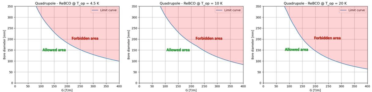
Fig. 6.1.27: A-G plot for quadrupoles built with REBCO and operated at 4.5 K, 10 K and 20 K.
