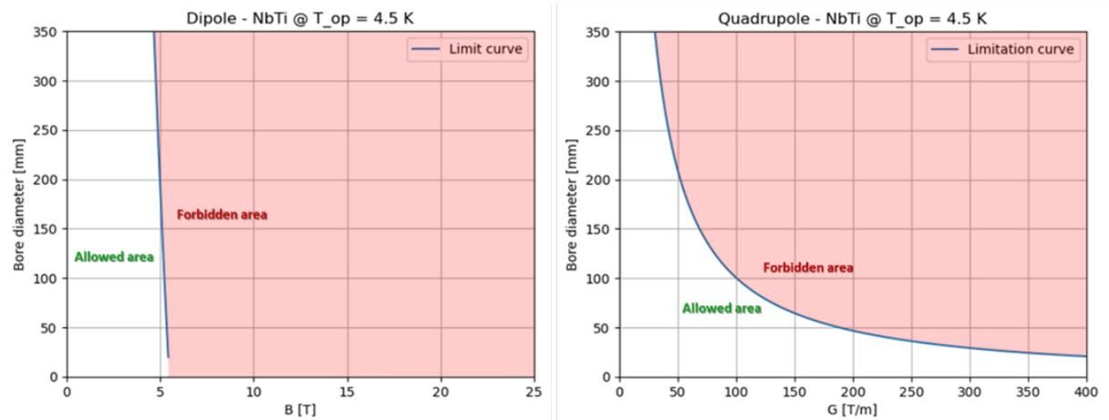
Fig. 6.1.28: A-B plot for dipoles and A-G plot for quadrupoles built with NbTi and operated at 4.5 K.
