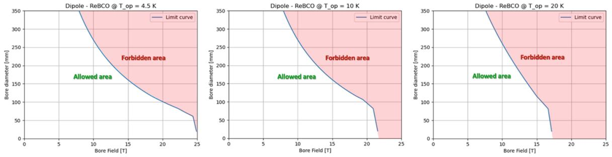
Fig. 6.1.26: A-B plot for dipoles built with REBCO and operated at 4.5 K, 10 K and 20 K.
