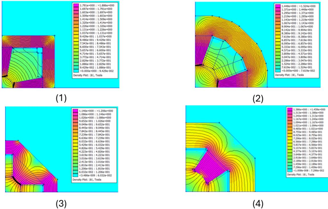
Fig. 6.1.23: Optimized quadrupole configurations for a bore aperture of 60 mm.
