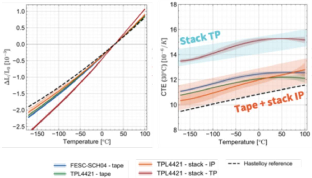
**Fig. 6.1.12:** Thermal contraction measurements of 2 ReBCO tapes (Theva TPL4421, and Fujikura FESC-SCH04) and of a soldered tape stack made with TPL4421. The measurements were carried out only along the In Plane (IP) direction for the tapes, while for the stack also the Through Plane (TP) measurements were performed
