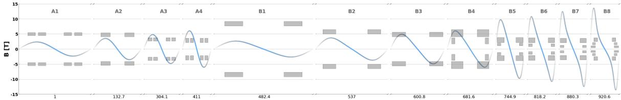
**Fig. 6.1.5:** Condensed schematic of the 12 types of cooling cells (A1 to B8) of a muon collider from the MAP configuration [300], with solenoid cross sections and the on-axis  $B_z$  field assuming each cell is in a lattice of neighboring cells of the same type.  $z$ -axis values shown correspond to the the middle of the first cell of each type.
