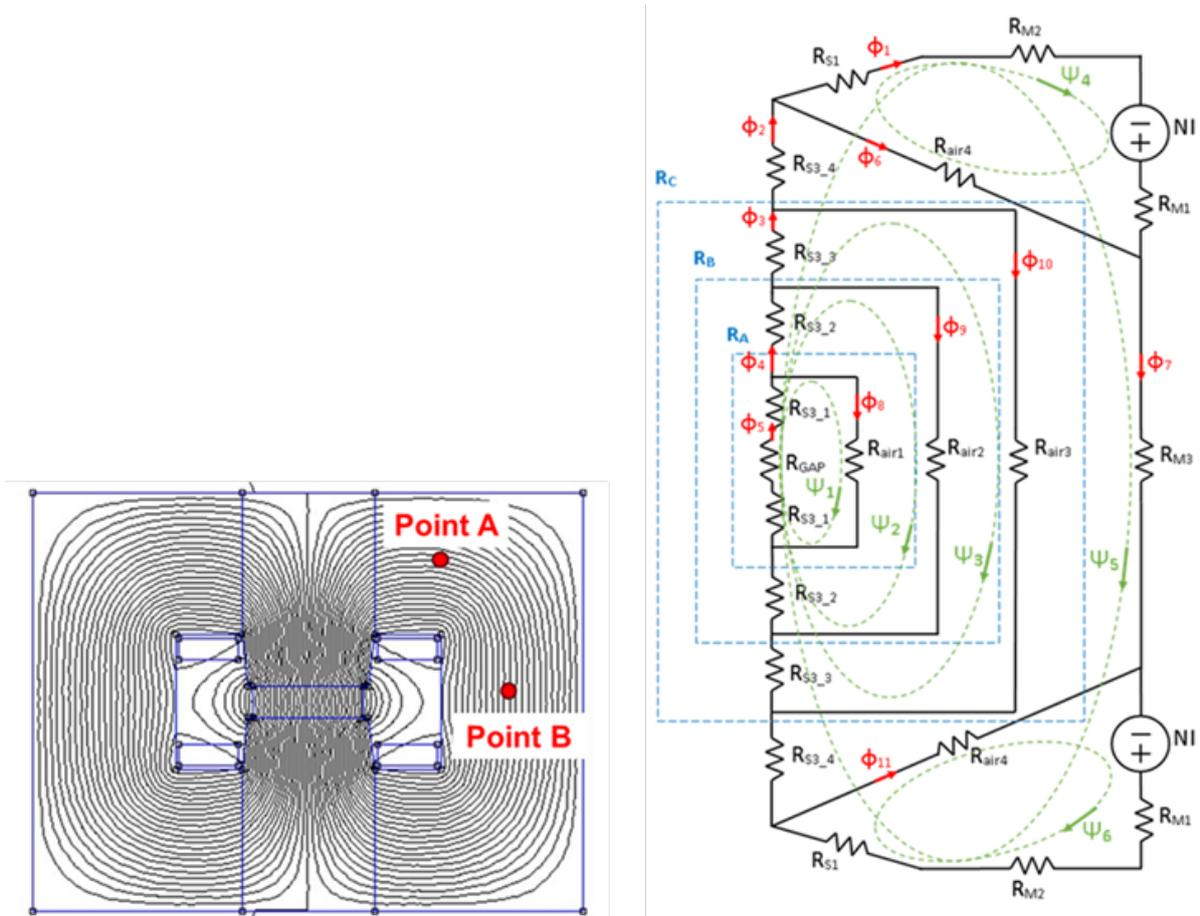
**Fig. 6.1.19:** a) Magnetic flux density map of the H-type dipole and b) corresponding equivalent magnetic circuit. The magnetic flux density calculated in Point A and Point B is used as a reference for the validation of the results of the circuit model.
