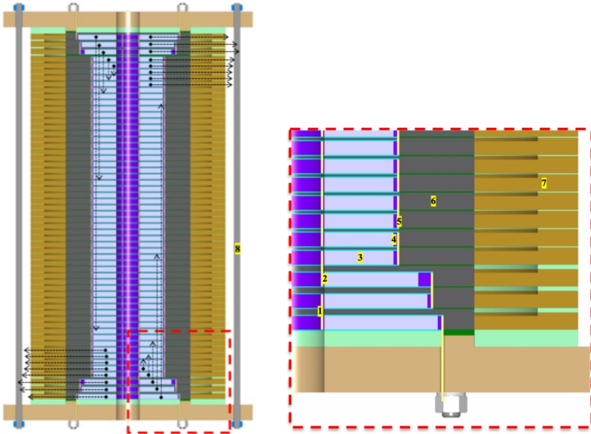
**Fig. 6.1.7:** Cross-section of the 40 T solenoid; the arrows indicate the axial and radial Lorentz forces acting on each pancake. The lengths of the radial arrows have been scaled down by a factor of 3.
