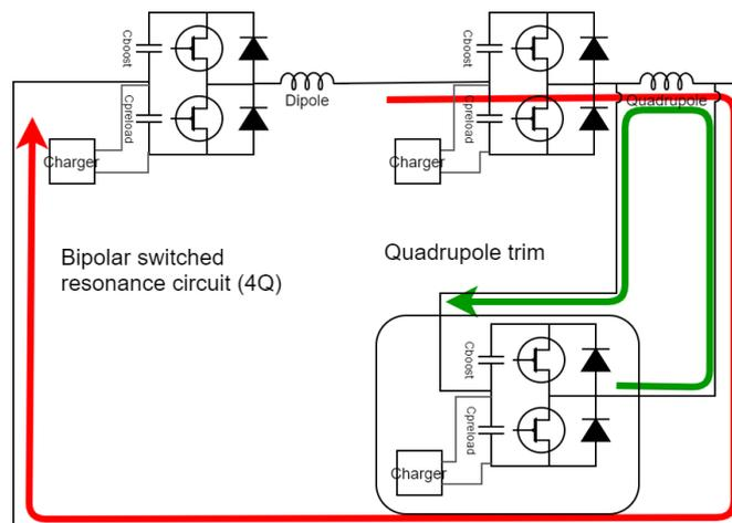
3376 **Fig. 6.2.1:** Possible quadrupole powering concept
