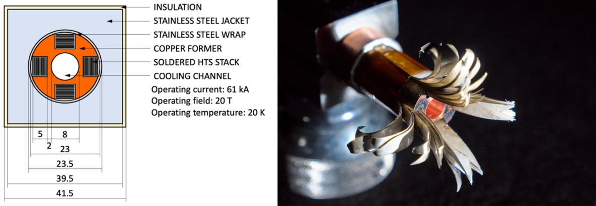
**Fig. 6.1.2:** Schematic view of the conductor configurations selected for the solenoid coils of the target, decay and capture channel (left) [329], with an image of a mock-up produced on real size (right) showing the HTS tapes, central copper former and jacket.
