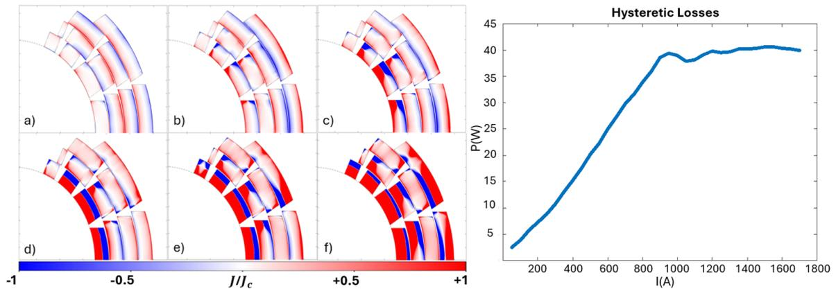
**Fig. 6.1.32:** Distribution of the current density in the coil cross-section at different step of the powering cycle and corresponding hysteretic losses profile as function of the magnet operating current.
