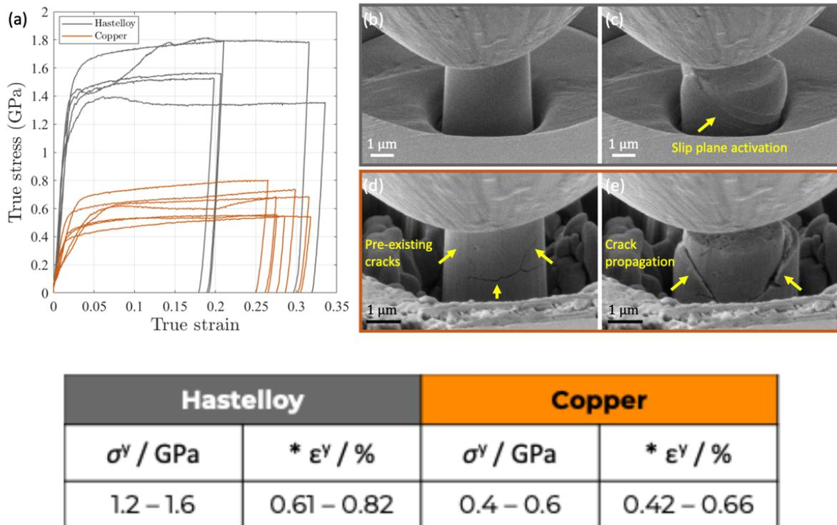
**Fig. 6.1.10:** (a) True stress-strain curves of Hastelloy and copper layers obtained by micropillar compression. (b)-(c) SEM images of a representative Hastelloy pillar before and after compression, respectively. (d)-(e) SEM images of a representative copper pillar before and after compression, respectively. The measured values are summarized in the table.
