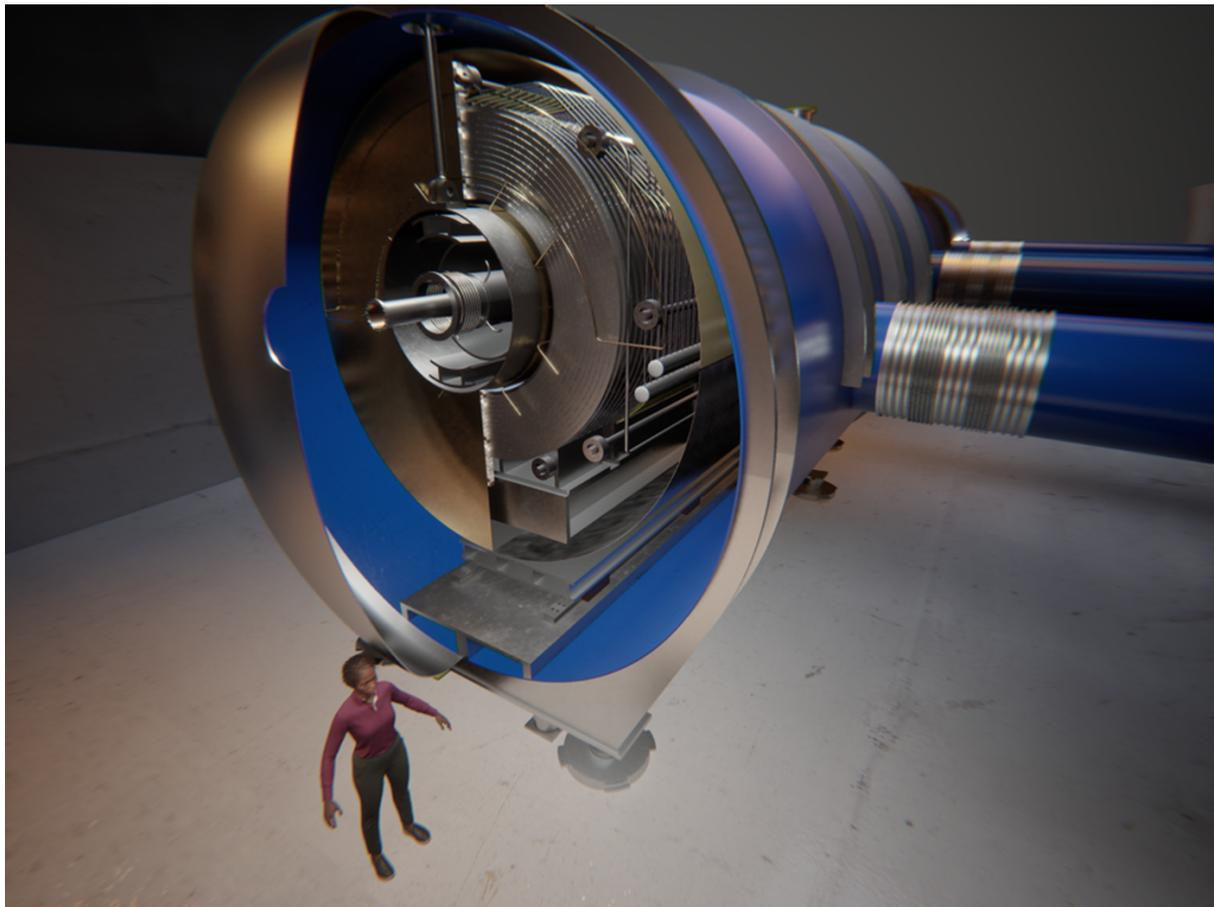
**Fig. 6.1.3:** Rendering of the magnet system for the target, decay and capture channel integrated in the cryostat, showing details of the winding, joints, cooling channels, thermal screen and supports.
