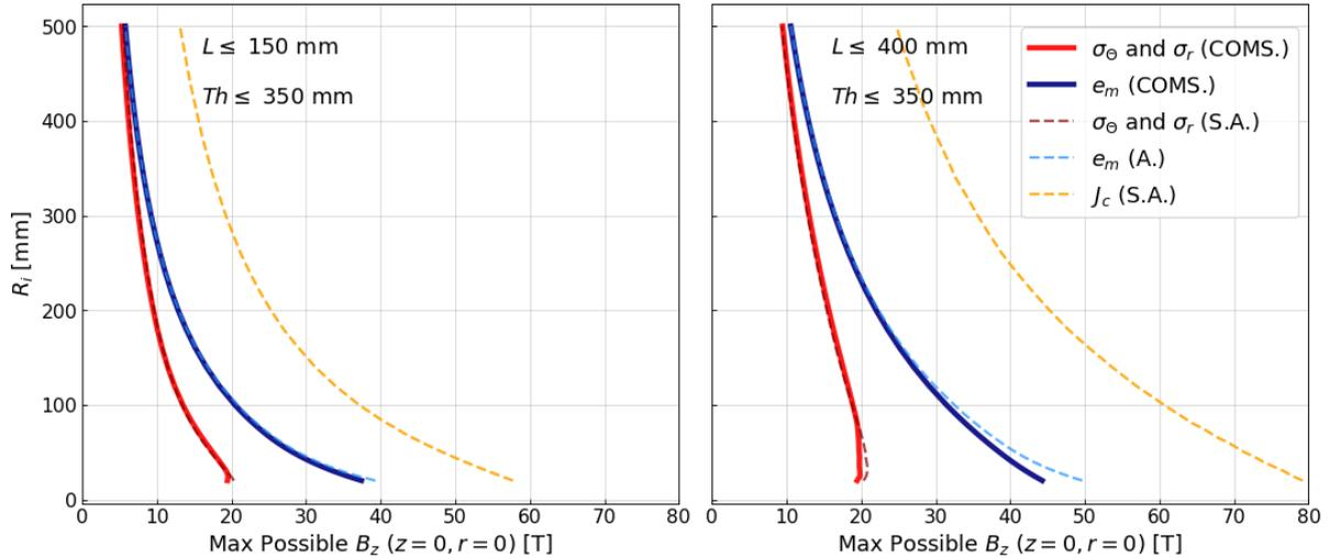
**Fig. 6.1.6:** The approximate maximum possible  $B_z$  on-axis versus bore radius ( $R_i$ ) of a single solenoid with a maximum thickness of 340 mm and a length up to 150 mm (top) or 400 mm (bottom), for different limiting parameters: red curves correspond to stress limits, blue to the magnetic energy density limit, and orange to the critical current density. Solid lines correspond to results found numerically with COMSOL (COMS.), and dashed lines to analytic or semi-analytic Eqs.
