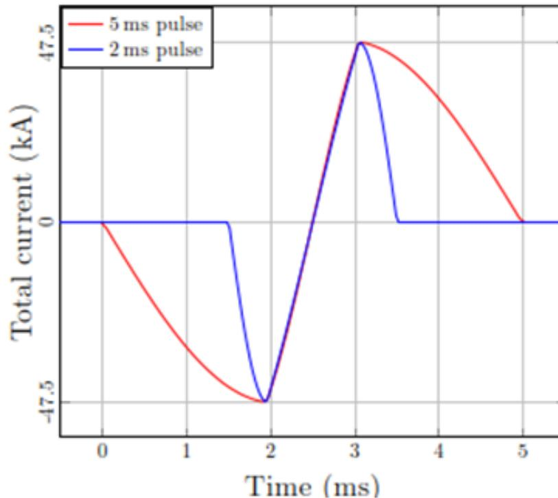
**Fig. 6.1.15:** Resonant current pulse for dipole magnets
