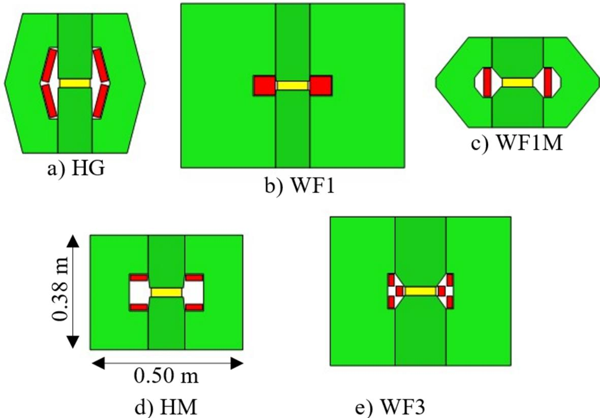
**Fig. 6.1.18:** Summary of the optimized geometries (the cross sections are to scale): a) Hourglass,  $J = 10$  A/mm<sup>2</sup>, b) Window-frame WF#1,  $J = 10$  A/mm<sup>2</sup>, c) Window-frame WF#1M,  $J = 20$  A/mm<sup>2</sup>, d) H-type HM,  $J = 20$  A/mm<sup>2</sup>; e) Window-frame WF#3,  $J = 20$  A/mm<sup>2</sup>.
