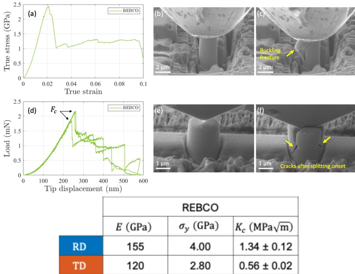
**Fig. 6.1.11:** (a) True stress-strain curve obtained by compression of a REBCO micropillar. (b)-(c) SEM images of the REBCO pillar before compression and after the first fracture, respectively. (d) Load-displacement curves obtained from splitting REBCO micropillars. (e)-(f) SEM images of a representative REBCO pillar before splitting and after the first fracture, respectively. The measured values are summarized in the table.
