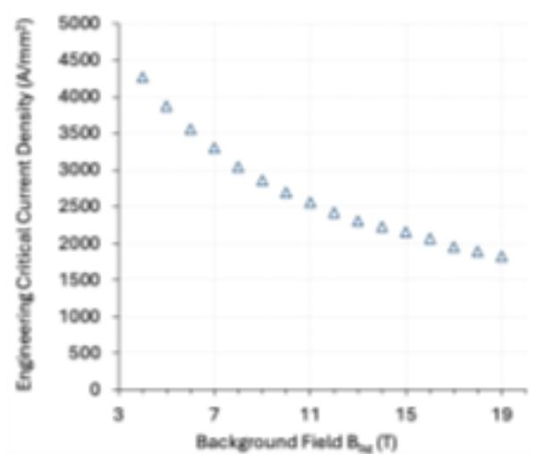
**Fig. 6.1.8:** Critical current measurements (triangles) at 4.2 K of a procured ReBCO tape ( $B \parallel c$ -axis).
