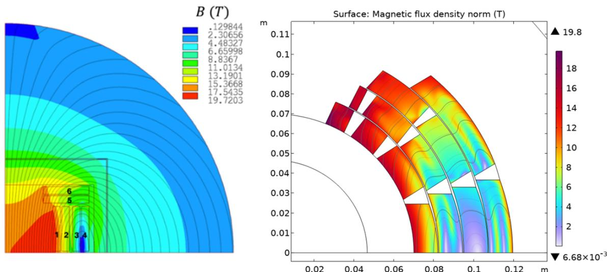
Fig. 6.1.30: Design of the cross section of HTS dipoles.
