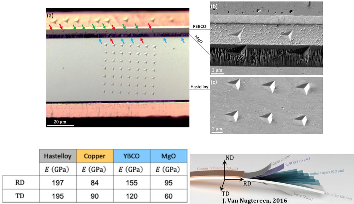
**Fig. 6.1.9:** (a) Optical image of the residual indentation imprints in the Hastelloy, copper, MgO (blue arrows) and REBCO (green arrows) layers. Red arrows indicate tests rejected due to being too close to other layers because of poor targeting. (b) SEM images of the residual indentation imprints in the REBCO and MgO layers. (c) SEM images of the residual indentation imprints in the Hastelloy layer. The measured values are summarized in the table.
