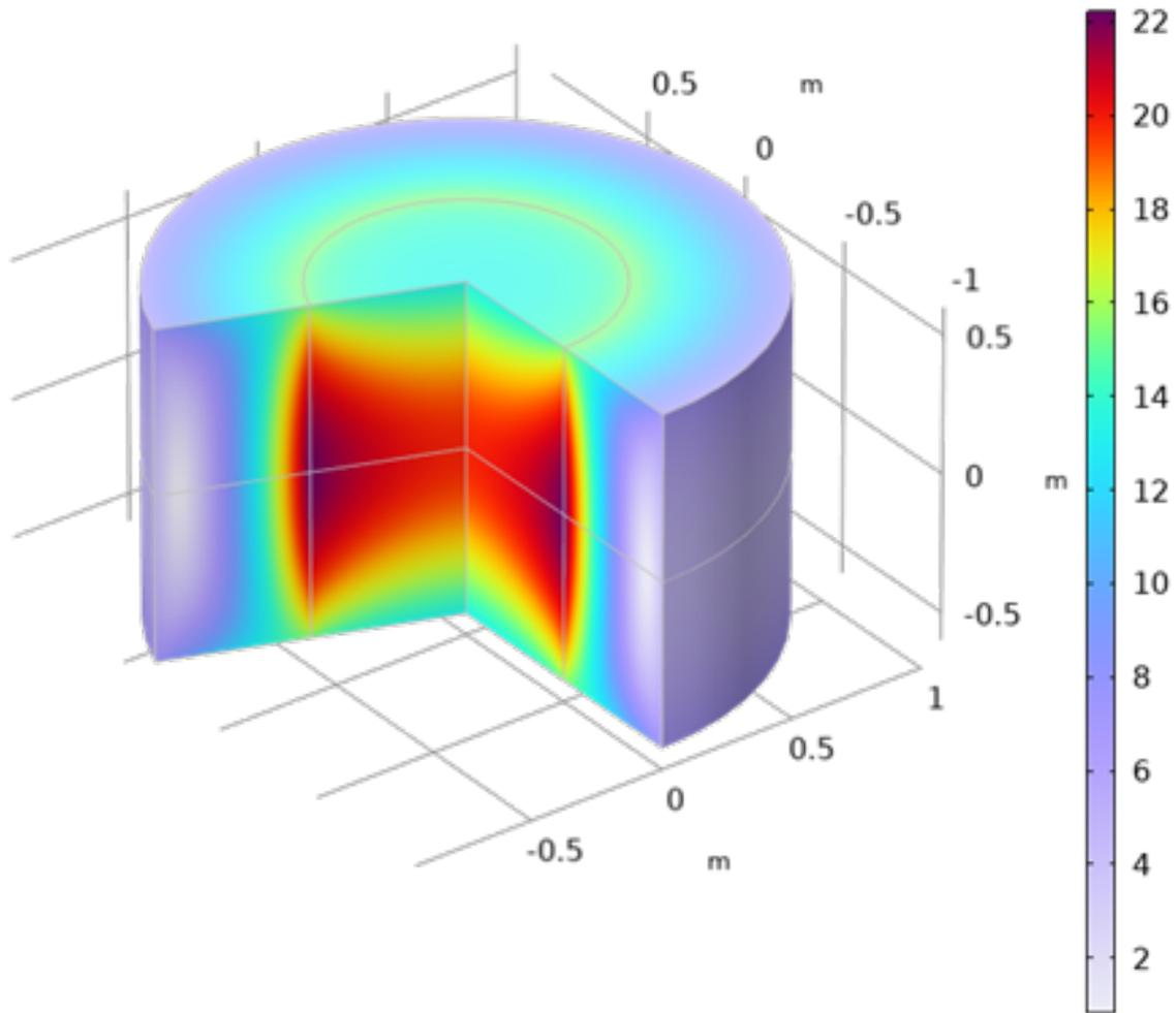
**Fig. 6.1.4:** A first result of configuration optimization for the design of a Target Solenoid Model Coil (TSMC) and corresponding field map in nominal operating conditions.
