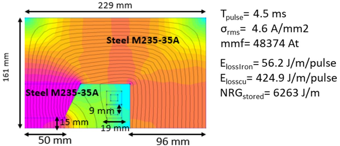
Fig. 6.1.21: Result of CAPEX+OPEX optimization on the dipole
