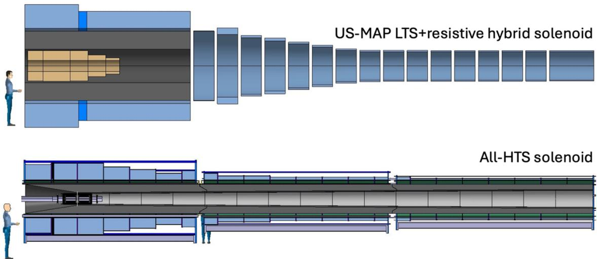
**Fig. 6.1.1:** Comparison (to scale) of the solenoid coils of the target, decay and capture channel of a Muon Collider, as produced by the MAP study (top) [294] and resulting from the optimization of an all-HTS solution (bottom) [328]
