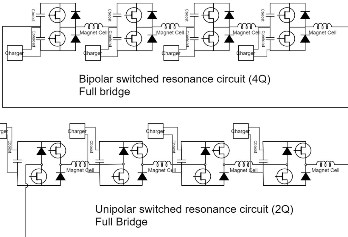
**Fig. 6.1.14:** Bipolar and Unipolar switched reluctance circuits
