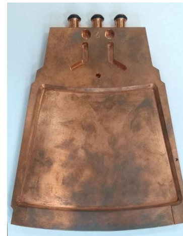
Target (back): Copper with microchannel cooling back
