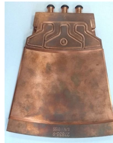
Target (front): copper blank. A ~ 300 \mu\text{m} of natural lithium coating typically present.
