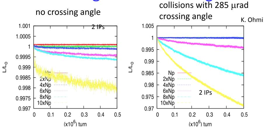
simulated luminosity lifetime with no crossing angle is 10 times better than with 285  $\mu$ rad angle ( $\phi \approx 0.65$ ,  $\beta *=0.55$ m,  $\gamma \epsilon=3.75$   $\mu$ m, E=7 TeV)
