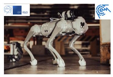
Develop legged ground robotic platforms for the autonomous and on-demand inspection, patrolling all the walkable areas. These robots are characterized by a high payload, allowing them to be equipped with a wide variety of sensors, and an enhanced mobility, which makes them suitable to operate inside detector cavern.
