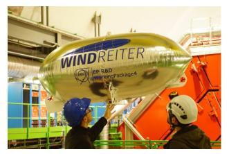
Develop Lighter than Air Unmanned Aerial Vehicles (LtA UAV), such as blimps, to provide a 3D environmental mapping of the background magnetic field and radiation dose of the whole cavern volume by employing a custom lightweight payload. Blimps are harmless solutions for the detector equipment in case of failure.
