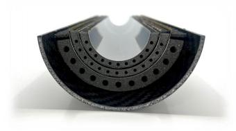
Develop new wafer-scale curved silicon pixel chips to surround the beampipe and their carbon foam mechanical support. This concept has the potential to reduce the material budget and to bring the first detection layer closer to the interaction point.
