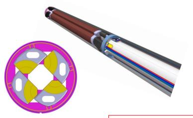
Development of a retractable Vertex Detector, inside the beampipe, positioning the first sensor layer as close as possible to the interaction point. Apertures, impedance and vacuum stability are key beam parametres and the Vertex detector petals has a direct impact on them.
