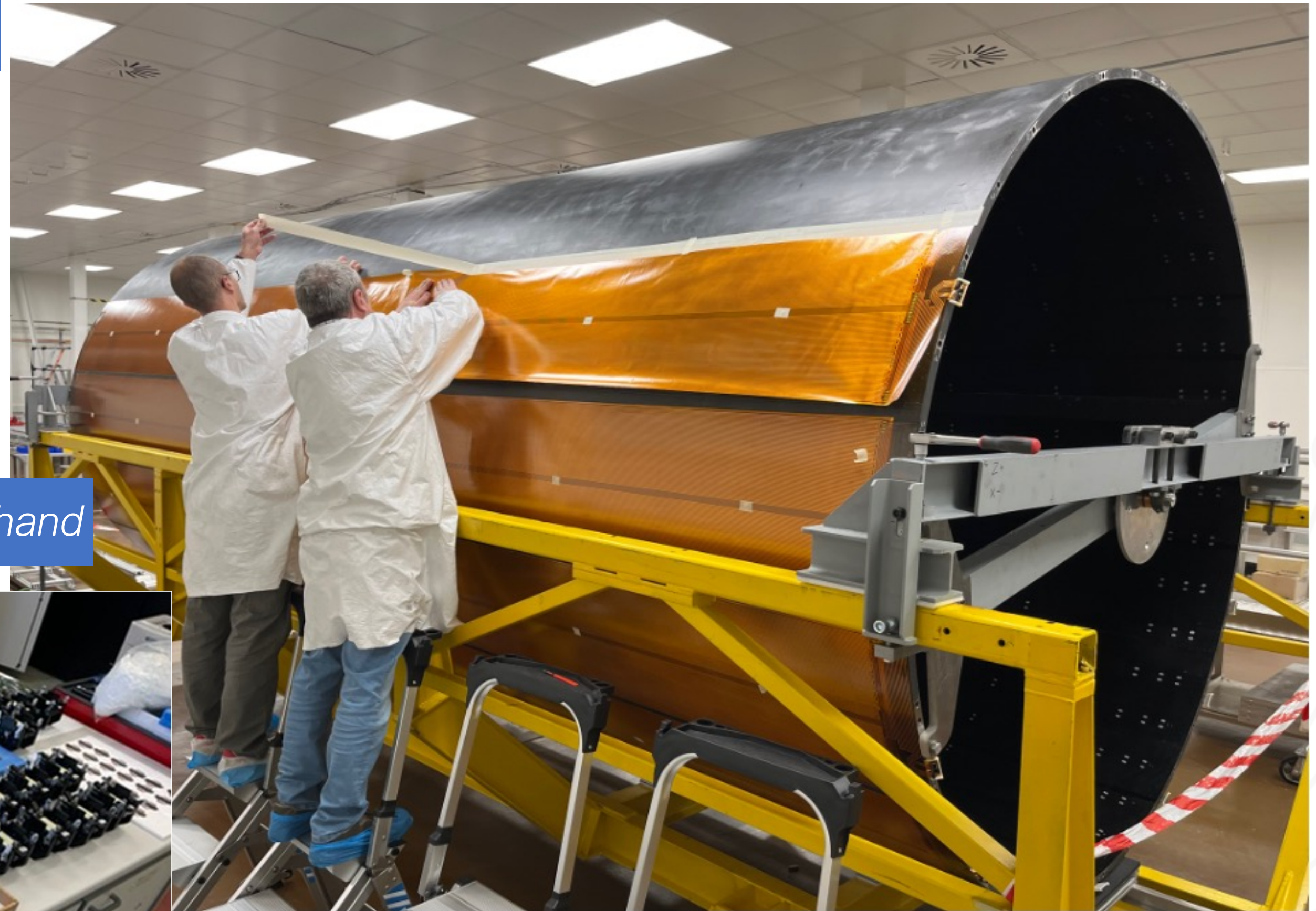
BTL-Tracker Support Tube heating foil gluing Ready for BTL installation early March
