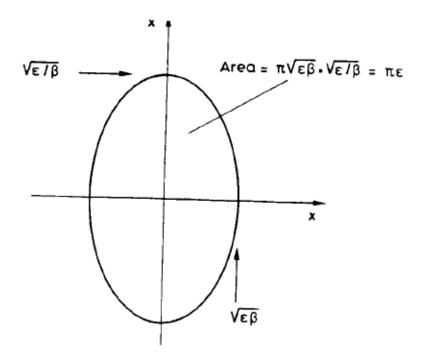
The area within the contour is proportional to the emittance of the beam. At constant energy we express this as the area  $\varepsilon = \int y' dy$  in units of  $\pi$ .mm.milliradians. We have shown
