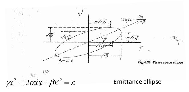
For plasma sources the ion temperature and source outlet aperture give the minimum emittance.
