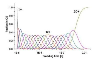
Charge state evolution for Ti<sup>+</sup>-ions in an EBIT with a current density of 10<sup>4</sup> A/cm<sup>2</sup> and an electron energy of 5 keV.
