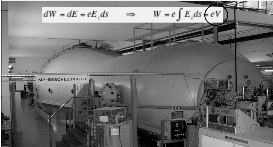
Electro Static Accelerator: 12 MV-Tandem van de Graaff Accelerator at MPI Heidelberg
