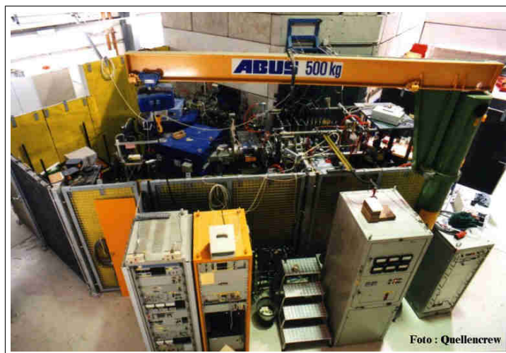
Figure 1: Ion source, beam line with mass separation, and entrance into a linear accelerator.
