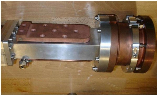
Matching transformer coupled to the plasma chamber
