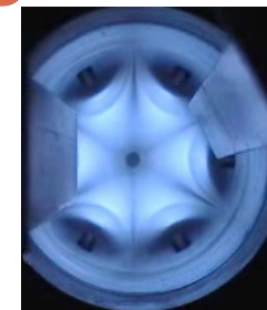
Photo of ECR plasma from injection (all thickness is superimposed => 6 lines) 10+14 GHz heating
