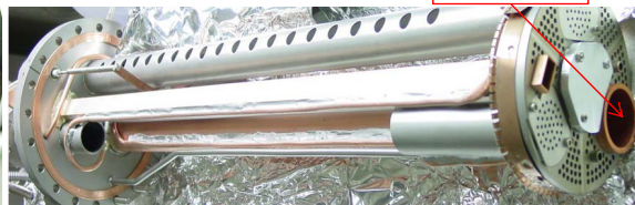
Removable UHV Injection system with 18+24 GHz
