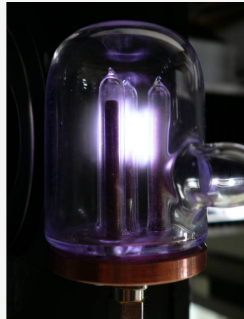
Distribution of light in a Xenon discharge (2 W) between the central antenna and the coupler with quasi-coaxial geometry p \sim 10^{-2} \text{ mbar}
