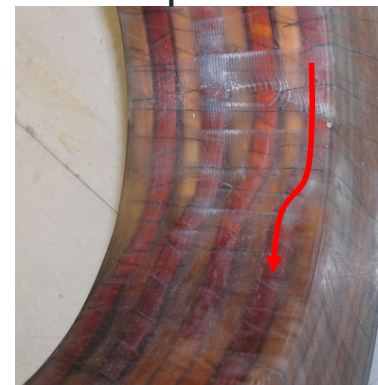
Passing from inward spiral to outward spiral, keeping same direction of coil rotation
