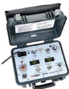
Current limited test of insulation
