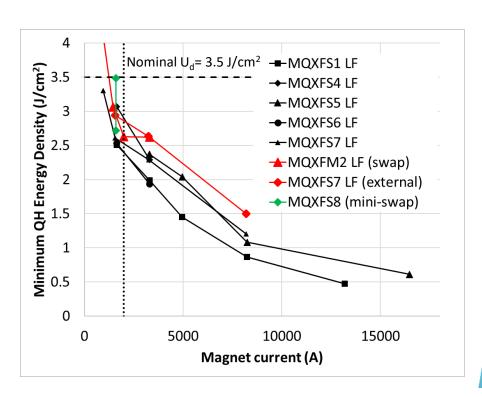
Minimum Energy Density =  $2.5 - 2.7 \text{ J/cm}^2$  (to initiate a quench at 2 kA) Final QH configuration:
