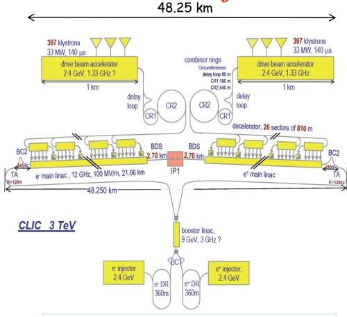
Overall layout Colliding energy of 3 TeV High acceleration gradient (100 MV/m)
