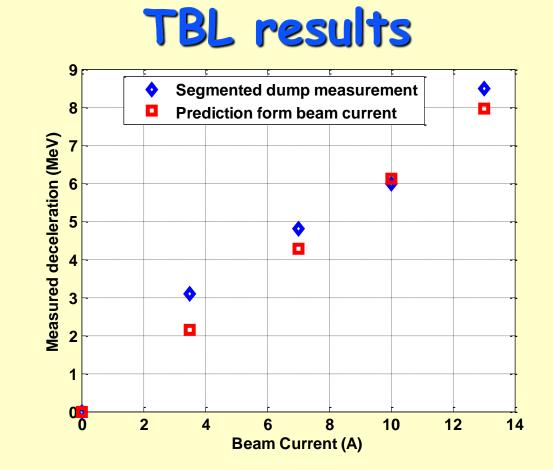
Have to assume 119 MeV initial energy, 117.5 measured  $\rightarrow$  1% error Form factor for predictions with current F=0.8 used To make the prediction from power fit, need to assume 10% calibration error
