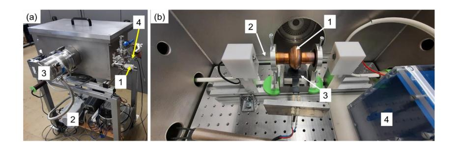
Flash lamp annealing system for the high temperature treatment of 6 GHz or 1.3 GHz cavities. (a) shows the external view of the FLA chamber. 1 and 4 shows the electrical connections to the Xe-lamp and preheating system, respectively, while 2 and 3 are pre-vacuum and turbo -molecular pumps, respectively. (b) shows inner view into the chamber. 1 is the 6 GHz cavity, 2 is the Xe-lamp, 3 is the preheating plate and 4 is high voltage ignition system for the Xe-lamp.
