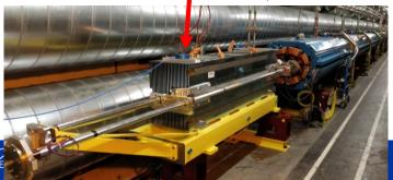
Power deposition in magnets depends on collimator + mask locations
