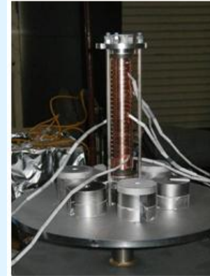
Pressure: 60 PSI (60 LB for this structure disks) Holding for 1 hour at 1020°C
