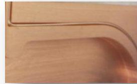
Brazing wire groove (Au/Cu 25/75)
