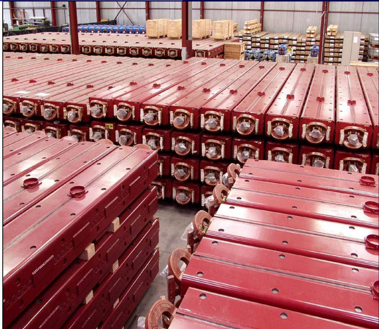
Dipole magnets waiting for installation
