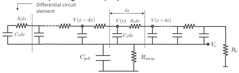
The propagation of the signal generated by a charge deposited at the resistive strip surface is described by the following expression.
