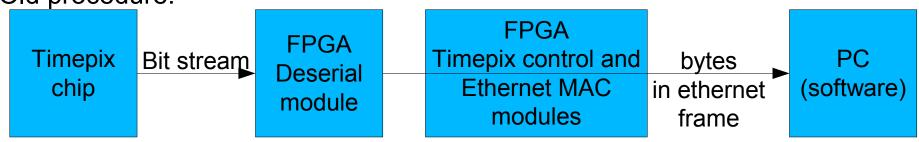
Only pipeline data: Convert bit stream to bytes for ethernet
