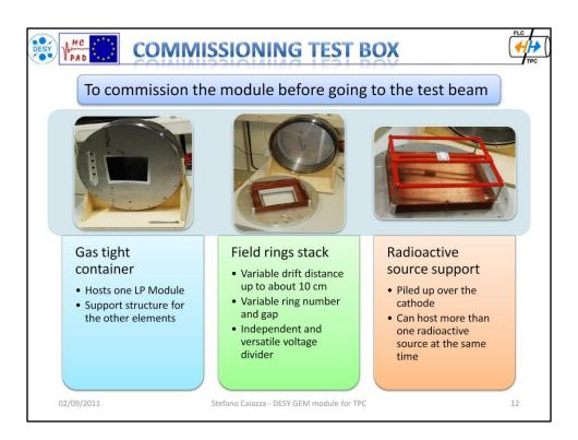
Another thing we were doing this last year, was the development of the text box for the module commissioning. The idea was to use this device to test the module before going for a test beam. The testbox features 3 main elements:
