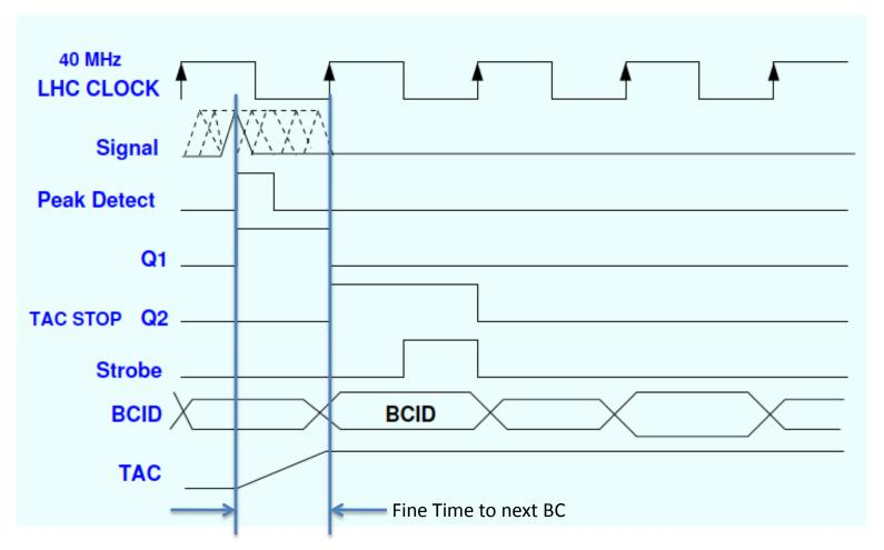
40 MHz BC clock convenient for LHC but any clock can be used to related hit with trigger accept
