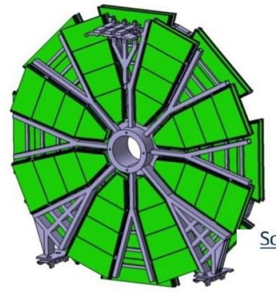
A tentative Layout of the New Small Wheels and a sketch of an 8-layer Chamber built of 2 4-layer multilayers separated by an instrumented Al spacer for monitoring in-plane alignment
