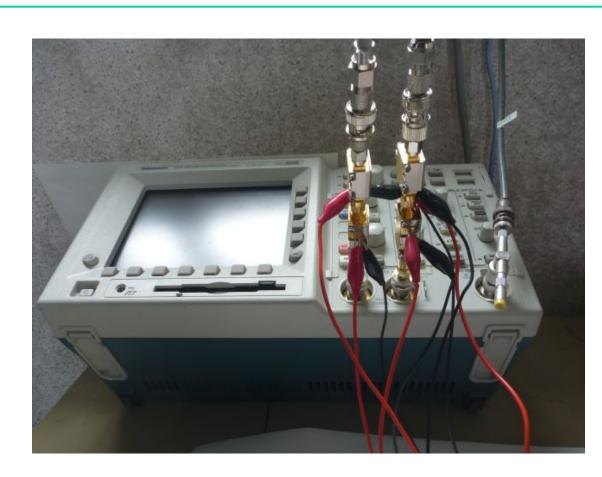
Outputs of the power detectors are recorded with a digital oscilloscope, TDS 3032 by Tektronix, Inc.. The oscilloscope is operated to record waveforms coincidently with event trigger signals from the air shower array. The record length per waveform is 10000 points with the sampling frequency of 0.1 GHz and the voltage range is -250 mV to +250 mV with 8 bit resolution. Each input is set to 50  $\Omega$  impedance and AC couple.
