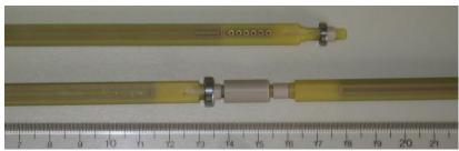
More precise measurement of the Field Quality will be provide by the NEW rotating coils system (Ø of 7.7 mm) under commissioning in these days (Special Thanks to Olaf Dunkel).
