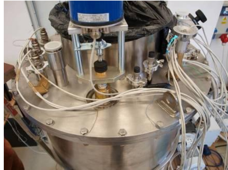
Top view of the cryostat with wiring
