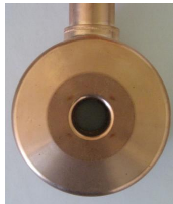
Sparking effects (@1.7kp) on Linac4 DTL prototype
