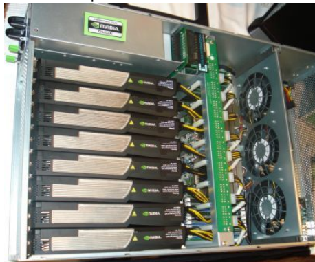
Server example with 8 Tesla GPUs
