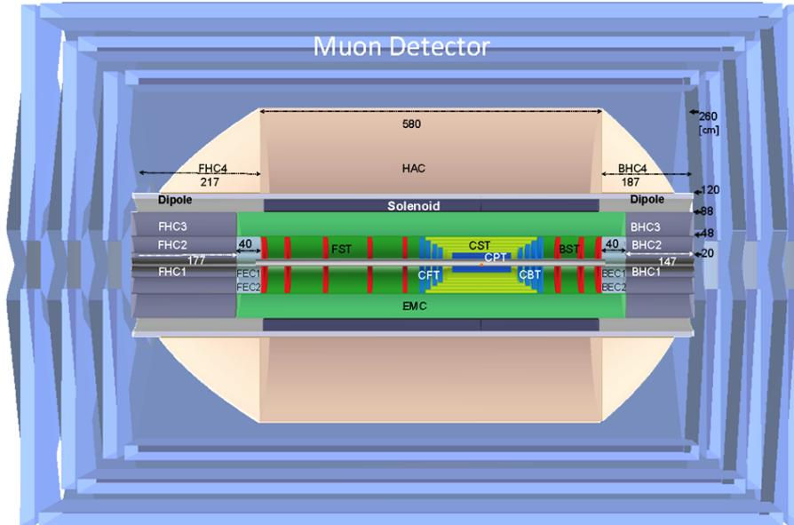
Figure 3: An  $rz$  cross section of the LHeC detector in its baseline configuration with the magnet configuration for LR with the solenoid and dipoles placement between the electromagnetic and the hadronic calorimeters. The proton beam, from the right, collides with the electron beam, from the left, at the IP which is surrounded by a central tracker system complemented by large forward and backward tracker telescopes followed by sets of calorimeters.
