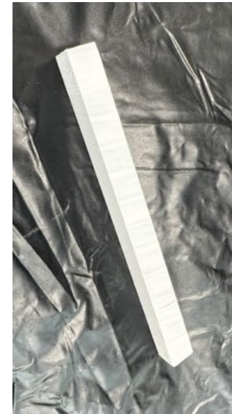
Wrapped with Teflon tape
