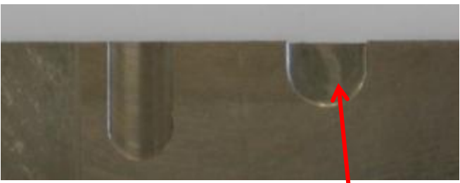
Very good result with a standard carbide tool
