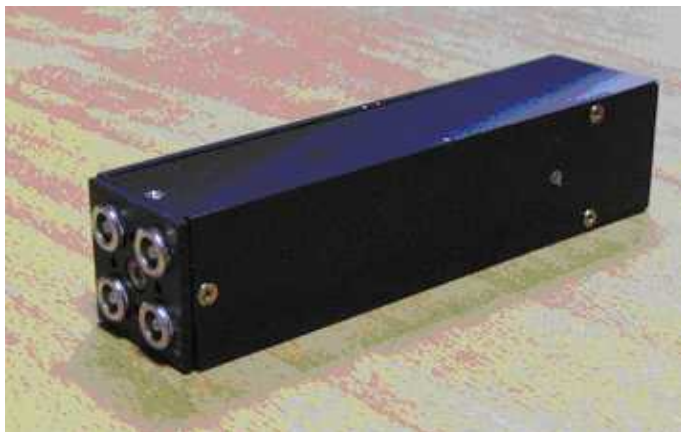
Cooled module with 4 SiPMs 5x5mm 2
