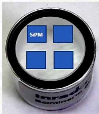
Stilbene with four SiPMs 6×6 mm 2 (SensL, J ser.)
