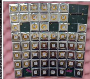
Scintillator tile module with trapezoidal tiles
