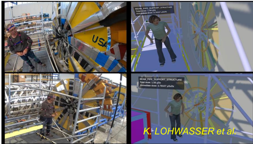
Dose estimation for decommissioning in ATLAS cavern (integration of FLUKA radiation maps, CAD models, and field-data acquired using motion caption system during mock-up tests in VR environment)
