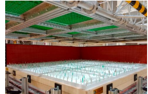
Installation of MPPC-PCB
