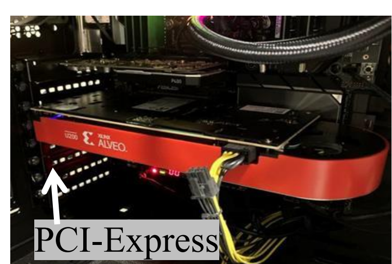
FPGA accelerator connected to PC via PCIe (Alveo 200 ©AMD)
