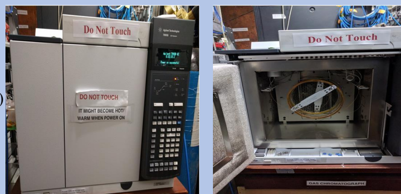
Agilent 7890B GC system used for the study. The gas chromatograph separates and quantifies gas mixture components with sensitivity in ~ ppm.
