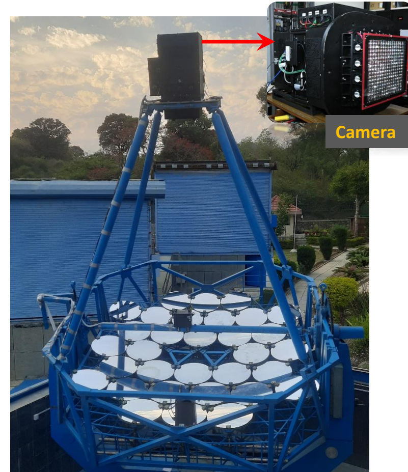
Camera mounted at focal plane of telescope
