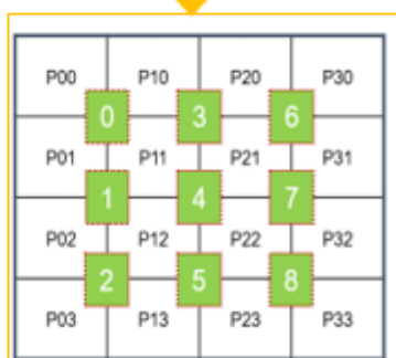
Full Trigger (4NCNN) in CDM, 9 combinations, Individual enable/disable control
