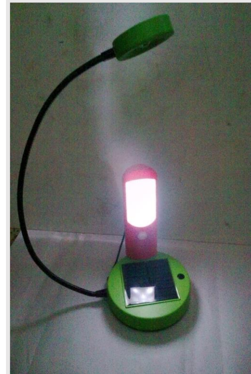
Demonstration of solar lamp with NPL anode & CECRI cathode
