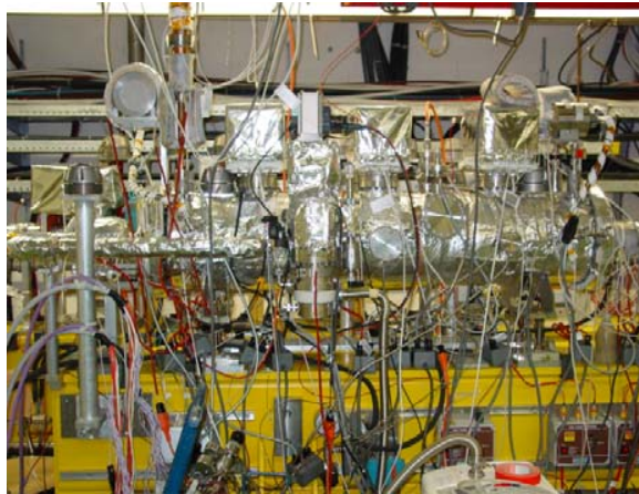
vacuum tanks containing Power Extraction Transfer Structure
