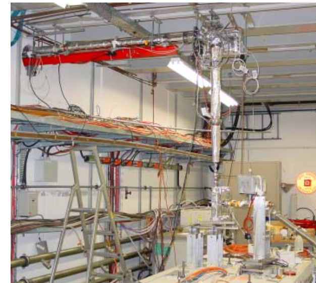
high power load / accel. structure
