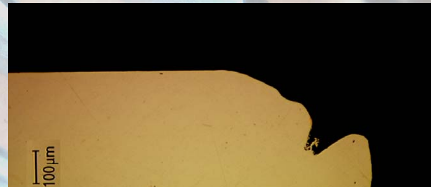
Damaged iris – longitudinal cut
